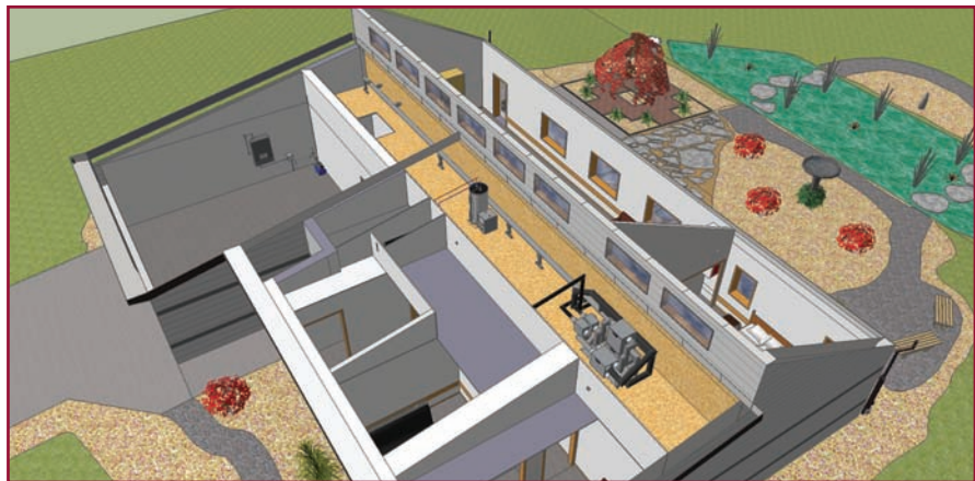
Figure 3: View of utility chase (attic) where the heat pump, fresh air ventilation system and the heat pump water heater are located.
