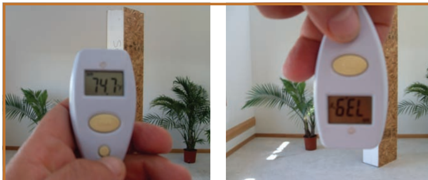
Photo 5: Equinox ceiling temperature and the temperature of the uninsulated concrete floor are shown on the handheld infrared thermometer display. It was a 91°F (33°C) day on Sept. 23, 2010 in Urbana, Ill.
