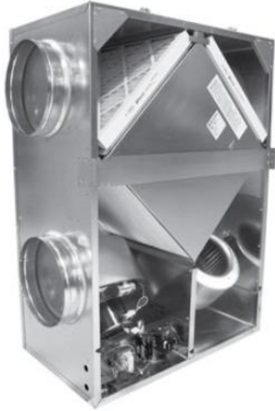
Figure D7 Renwaire HE1XINV energy recovery unit with 250 to 1100cfm air flow range. Unit dimensions 50" high by 36" wide by 24" depth.
