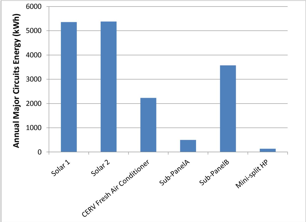
Figure 3 Major electrical circuit energy users in Equinox House.
