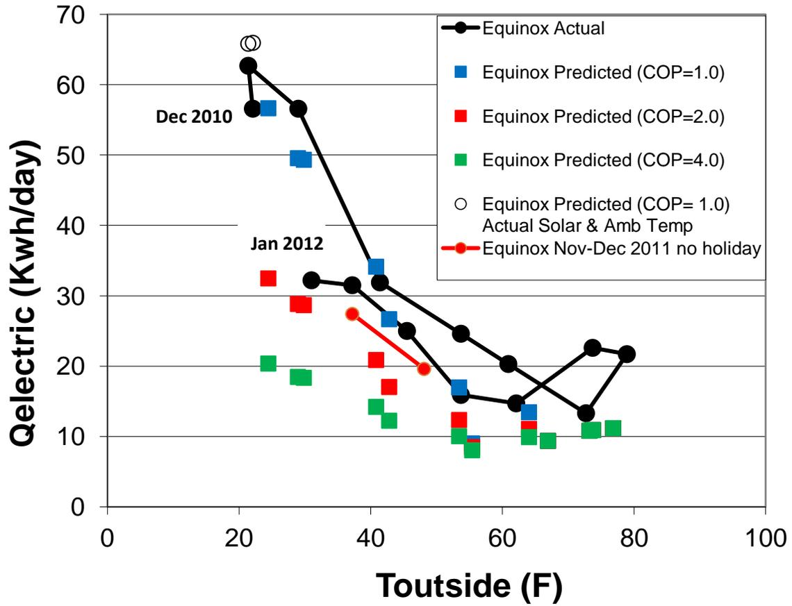
Figure 2 Actual Equinox House energy performance versus simulation model predicted energy performance for electric resistance heating (COP=1), mini-split air source heat pump (COP=2) and ground source heat pump (COP=4).
