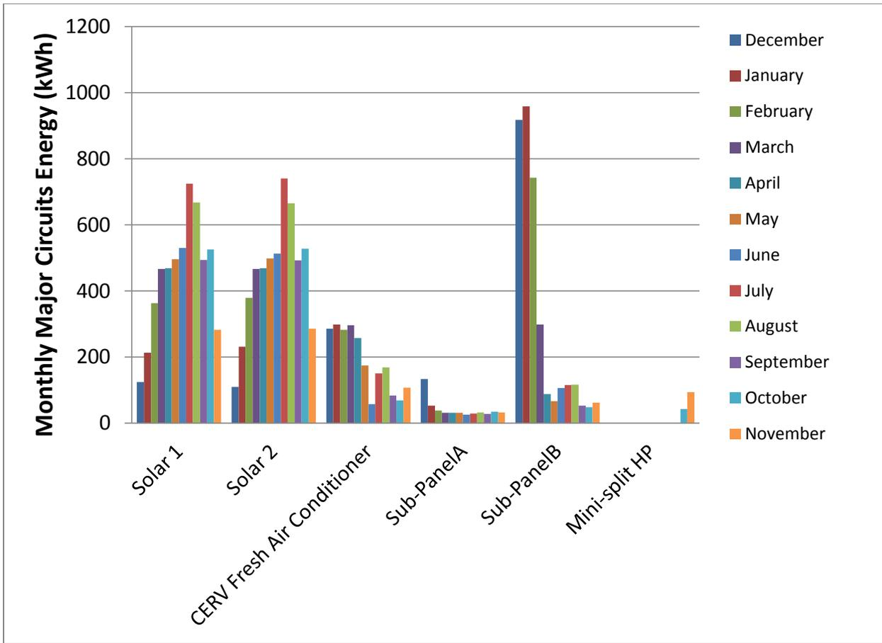
Figure 6 Monthly breakdown of major circuit energy.
