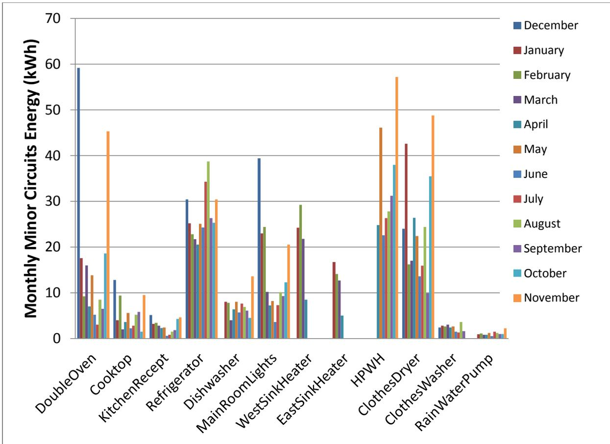
Figure 7 Monthly breakdown of minor circuit energy.
