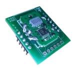
The outside VOC sensor option allows the CERV2 to measure VOC levels in the fresh air entering the CERV2 from outside. An Outside VOC Prevention function can be enabled by the user to allow the CERV2 to disable ventilation during times when the outside VOC level is higher than inside. This is especially useful in locations where wildfires or other outside pollutants are a concern.
