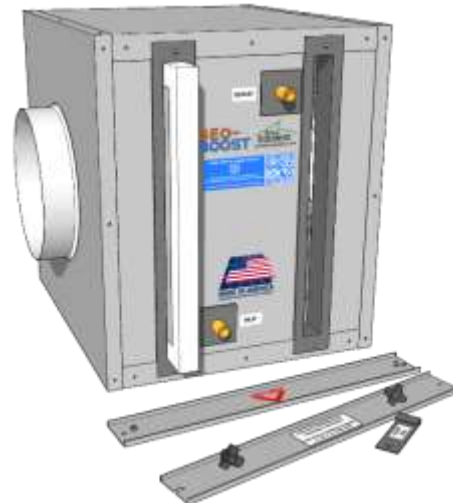
Reverse Filter direction and insert into Left slot
