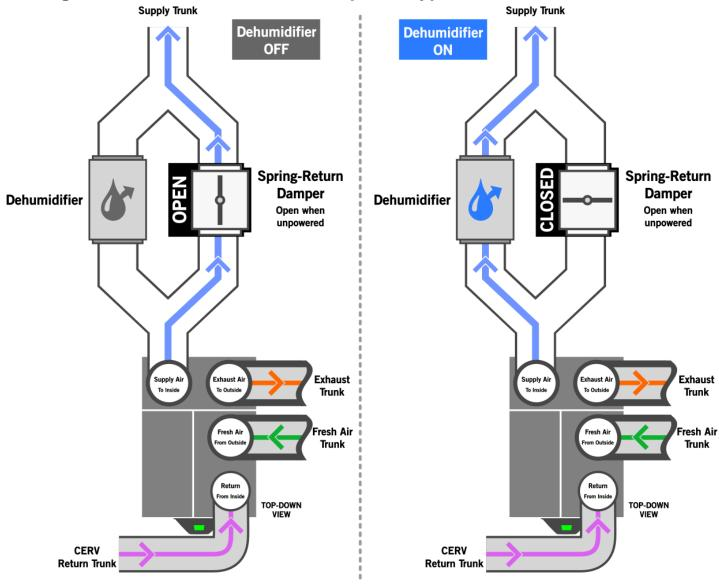
With a dampered bypass, airflow is allowed an unrestricted path when the dehumidifier is off (left image), but must pass through the dehumidifier when it is running (right image). To use this configuration, a **Power Close** spring-return damper should be used. The spring-return damper should be **open** when in an **unpowered** state, and **closed** in a **powered** state. See the Electrical section below for information regarding wiring connections to the damper.
