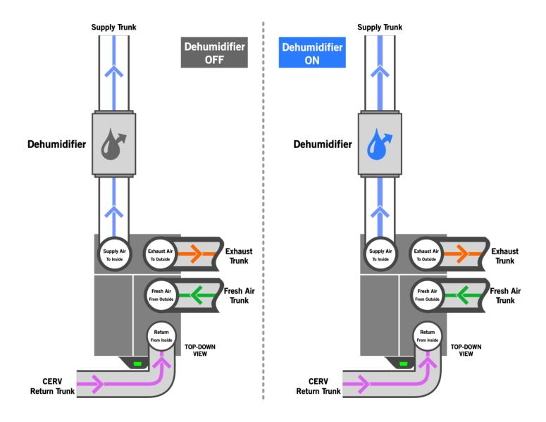
In this configuration with the dehumidifier directly inline with the Supply Air, the CERV will continue to push air through the dehumidifier even when the dehumidifier is not active. This may result in increased static pressure and therefore lower airflow for a given fan speed (and power). If this is a concern, the following design with a bypass may be used instead. See the Electrical section below for information regarding wiring connections to the damper.
