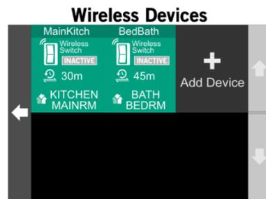
Pair wireless both switches, set the time length and fan speed (if desired). The first switch activates both Kitchen and Living room Zones, while the second activates the bedroom and bath.
