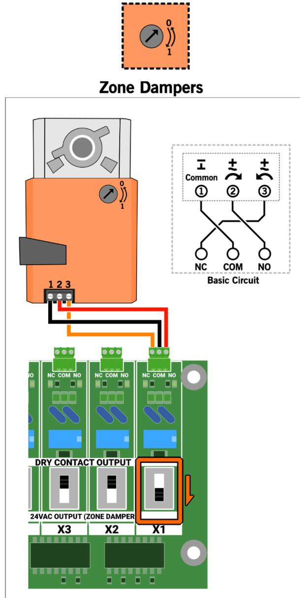
IO Expansion Board is capable of directly outputting 24VAC through its terminals without requiring connection to an external 24VAC source. NOTE: for this configuration, you must move the slide-switch above the terminal block towards the 24VAC OUTPUT label. LED indicators on the IO Expansion Board will light up above either the NO or NC terminals, to indicate which is active. Up to six zone dampers may be connected to the IO Expansion Board.
