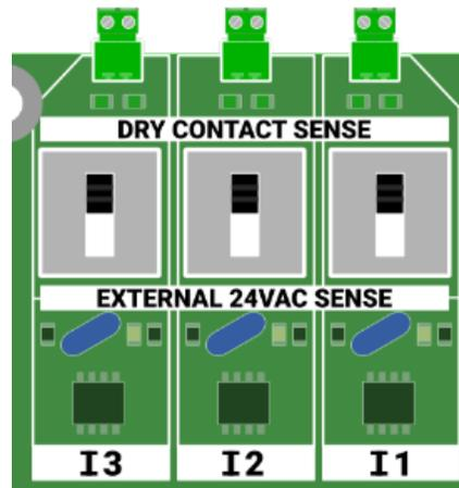
**Output channels** can be set to dry contact or 24VAC output. Set the toggle switch to the correct position for the output channels to be used and then make the proper wiring connections to the associated output channel screw terminals from the external auxiliary device.
