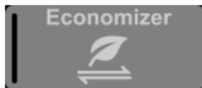
The CERV will not ventilate to help boost heating or cooling.
