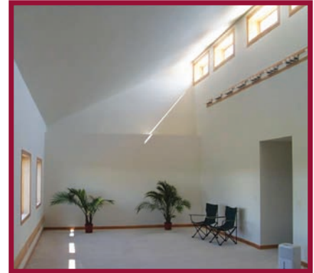
Photo 2: Interior light with full sun entering Equinox House on September 20. The sun's elevation through most of the winter will move the direct beam radiation onto the upper walls and ceiling.
