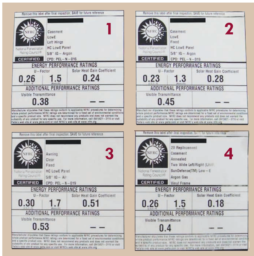
Figure 1: NFRC window performance parameters for the three types of windows installed in Equinox House and a replacement window installed in Newell Instruments Laboratory.
