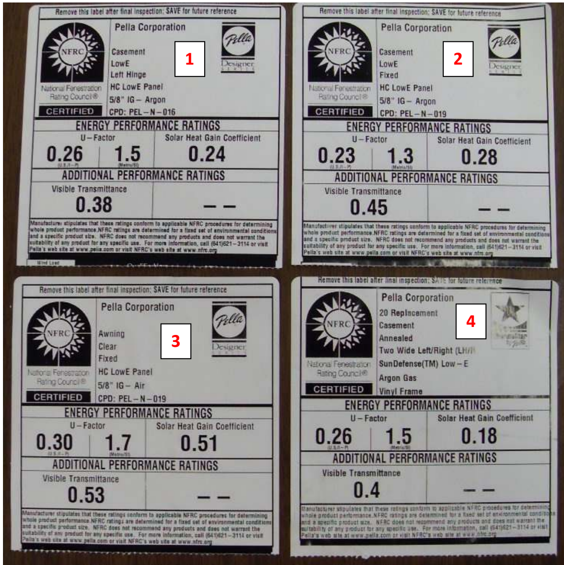
Photo of stickers removed windows we recently installed. Windows 1, 2 and 3 are used in Equinox House and window 4 was installed in Newell Instrument's Lab.
